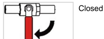
Ensure that the main isolation valve of the gas supply line is **closed** when the system is not in use for extended periods
