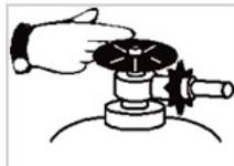
Ensure the cylinder valve is **closed** before removing the connecting hose or changing the gas cylinder
